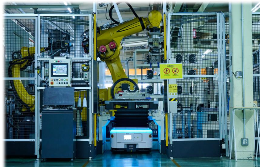
Automatic setup using in-house AMR and robots
