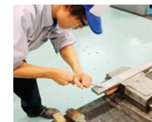
Surface finishing requires accuracy on the order of 1µm.
