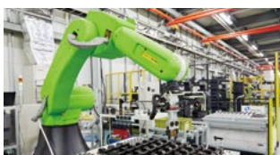
Automation using robots is advancing for sub-assembly work that involves a small number of parts and simple structures.
