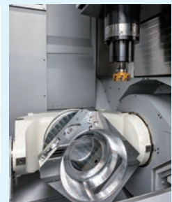
Simultaneous 5-axis machining and turning functions consolidate the machining processes for complex three-dimensional shapes.
