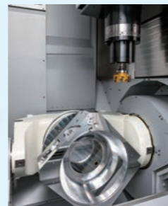
Simultaneous 5-axis machining and turning functions consolidate the machining processes for complex three-dimensional shapes.
