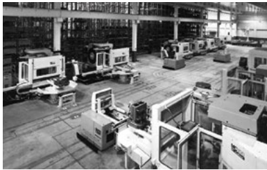
FMS factory at the Atsugi Plant (1983) Includes 10 machining centers, three automated guided vehicles, an automated warehouse, and tool stations.
