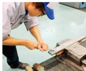
Surface finishing requires accuracy on the order of 1μm.
