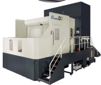
5-axis control Machining Center (D2)
